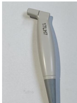
Figure 1: Hockey-stick transducer (17H7) compatible with TOSHIBA XARIO 200 Ultrasonography machine
